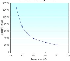
Fig.2 Viscosity profile of the resin/hardener mixture as function of temperature
